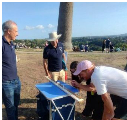
Image Left: Using Allan's spectroscope for observing the Fraunhofer lines
